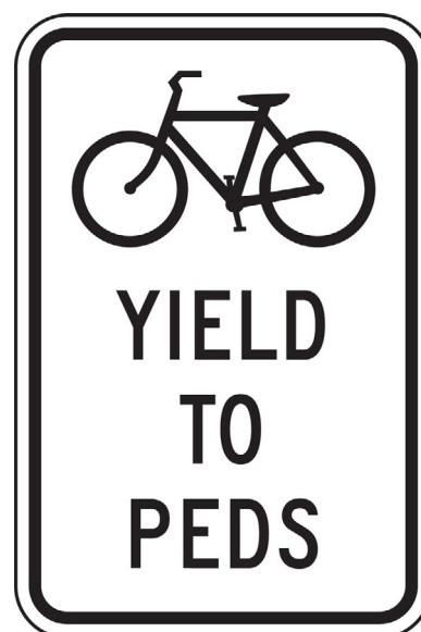
Figure 10: Signs can clarify yielding rules in shared use environments and may be modified based on expected user types.
